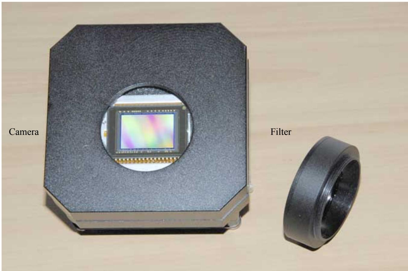
Just remove the filter like any other filter by unscrewing the nose piece anticlockwise
